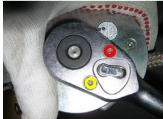
2. Place the rescue device and the pulley on „red“. Attach the rescue device to the chest of the safety harness.
